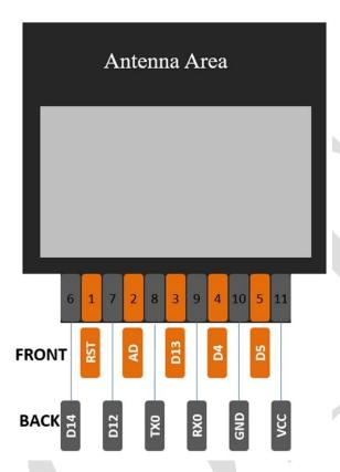
Fig. 2.1 ESP-02S Pins Definition
