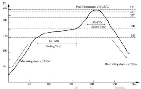
Fig.7.1 Recommended Reflow Profile
