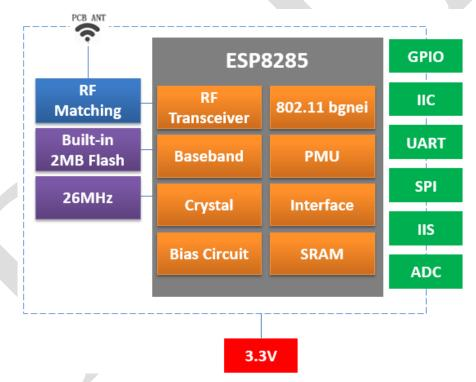
Fig. 1.1 ESP-02S Module Structure
