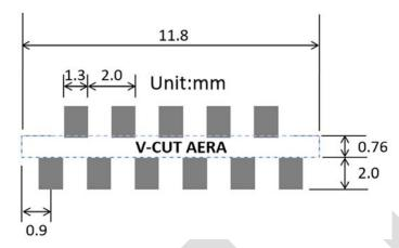
Fig. 3.3 PCB Layout for ESP-02S
