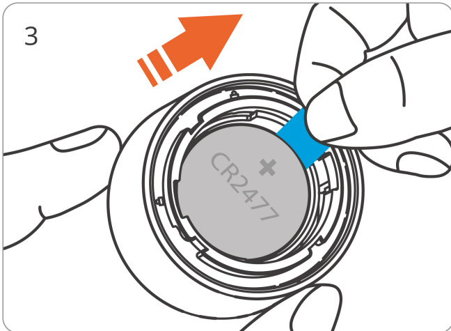
Take out the battery insulation sheet
